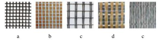
Textile Fiber Reinforcement: (a) carbon fiber textile;(b) glass fiber textile; (c) basalt fiber textile;(d) Polyphenylene benzobisoxazole (PBO) fiber textile; and (e)steel fiber textile.
